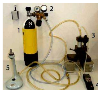
Figure 4. Measuring assembly for determining differential pressure in samples: 1 – pressure balloon with compressed air; 2 – pressure reducing valve; 3 – measuring chamber; 4 – differential pressure gauge; 5 – flowmeter.
