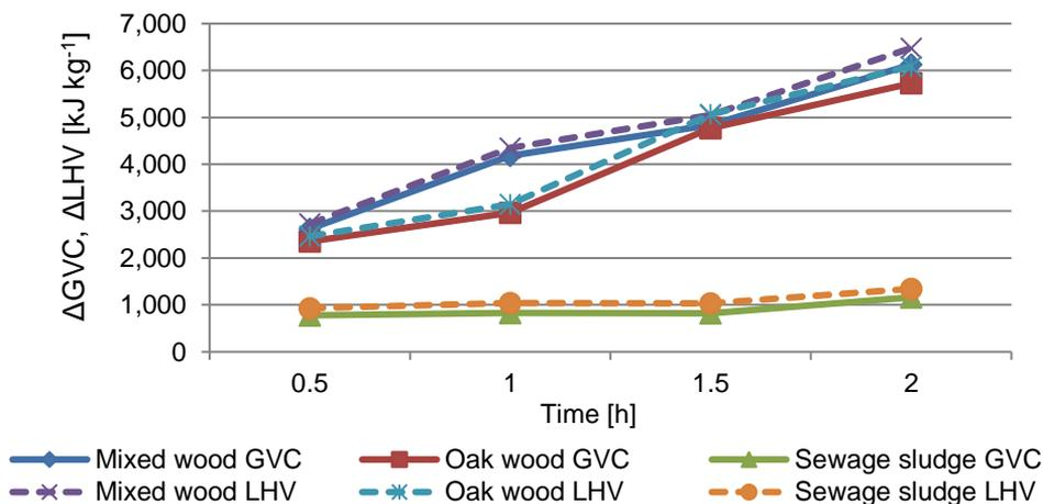
**Figure 6.** The difference in calorific value between torrefied material and raw material depending on operation time.
