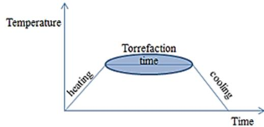
**Figure 1.** Schematic presentation of the process operation.
