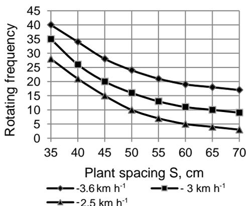
**Figure 4.** The dependence of the planting unit rotating frequency on plant spacing at different tractor gears.
