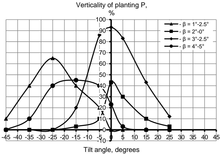
**Figure 9.** The dependence of planting verticality on the tilt angle of the planting cone β.
