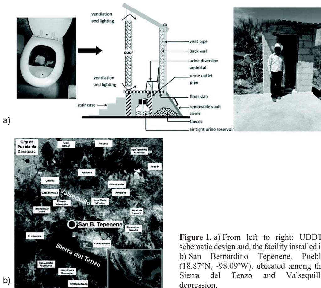
**Figure 1.** a) From left to right: UDDT, schematic design and, the facility installed in b) San Bernardino Tepenene, Puebla (18.87°N, -98.09°W), ubicated among the Sierra del Tentzo and Valsequillo depression.
