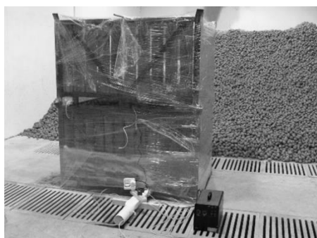
Figure 3. Storage boxes with ventilator and ozone generator during the storage period of ‘Dali’ potato tuber.
