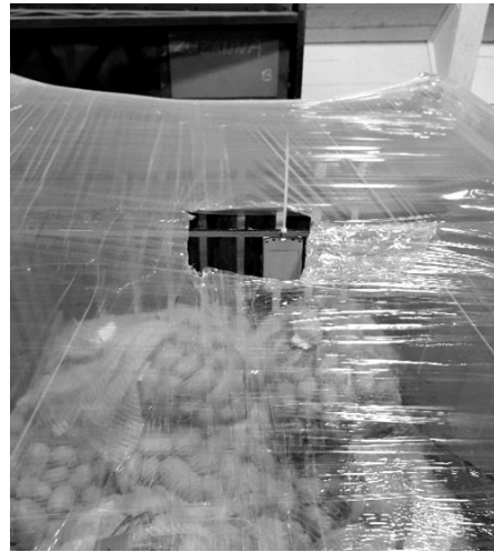
Figure 4. Datalogger placement in a storage box.
