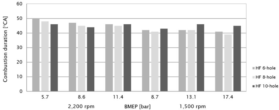
**Figure 8.** Combustion duration ( $^{\circ}\text{CA}$ ) at all engine loads, determined as crank angles between MFB 5% and MFB 90%.
