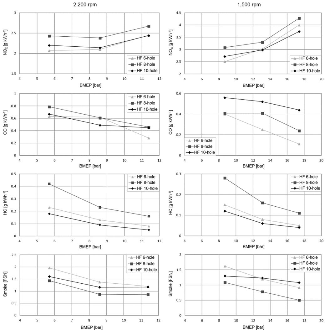
**Figure 9.** Brake specific emissions of NO<sub>x</sub>, CO and HC and smoke numbers versus engine load at two speeds.
