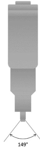
**Figure 1.** Spray angle schematics of the injector nozzles.
