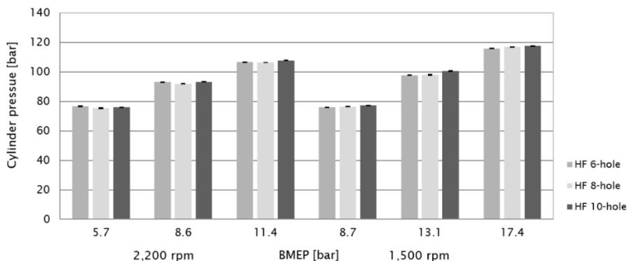
**Figure 5.** Maximum cylinder pressures at rated and intermediate speed with standard deviations.
