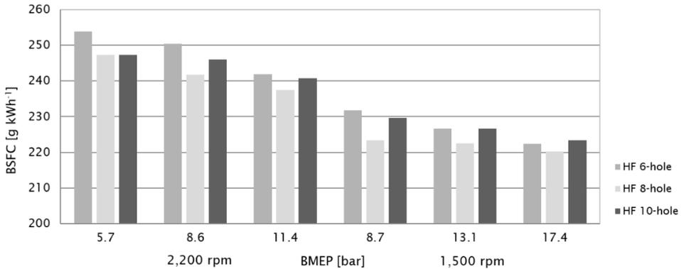
**Figure 3.** Brake specific fuel consumption at rated and intermediate speeds.
