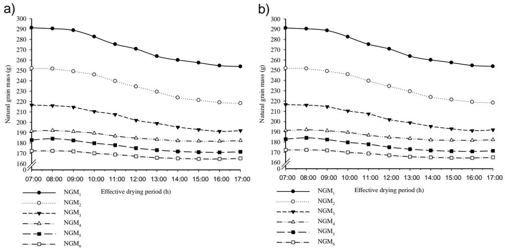
**Figure 10.** Reduction in the mass of a) natural and b) washed grains throughout the drying period: NGM<sub>n</sub> – Natural grain mass; WGM<sub>n</sub> – Washed grain mass; n – drying day.
