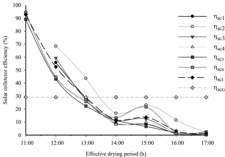
**Figure 5.** Thermal, instantaneous and global average efficiency of the solar collector throughout the drying period:  $\eta_{scn}$  – Solar collector efficiency; n – drying day; I – Instantaneous; G – Global.
