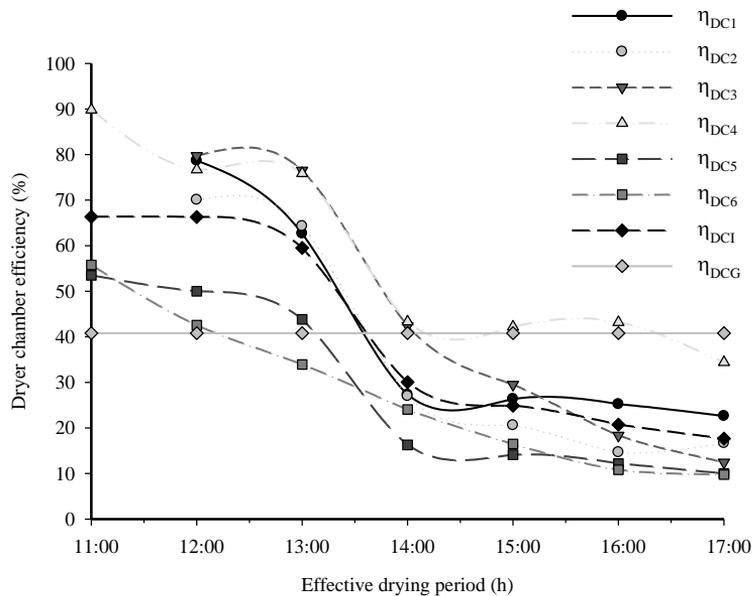
**Figure 8.** Thermal efficiency of the drying chamber of the hybrid solar-electric dryer over the drying period:  $\eta_{DCn}$  – Dryer chamber efficiency; n – drying day; I – Instantaneous; G – Global.
