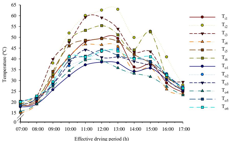
**Figure 6.** Temperature of the drying air in the SHSE chamber over the drying period: T<sub>n</sub> – Temperature; i – inlet; o – outlet; n – drying day.
