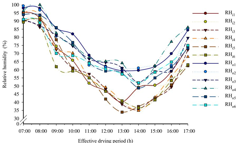
**Figure 7.** Relative humidity of the drying air in the SHSE chamber over the drying period: RH<sub>n</sub> – Relative humidity; i – inlet; o – outlet; n – drying day.
