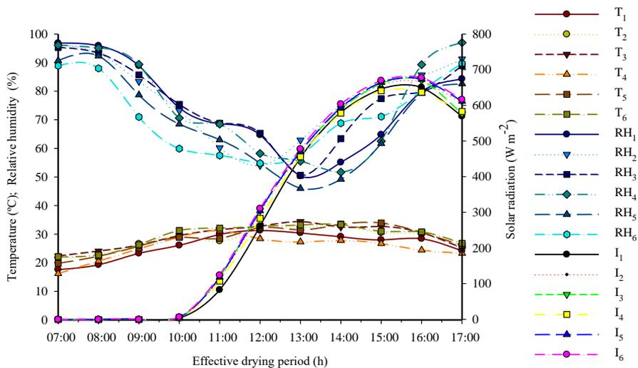
**Figure 2.** Temperature ( $^{\circ}\text{C}$ ), relative humidity (%) and global solar radiation ( $\text{W m}^{-2}$ ) over the drying period:  $T_n$  – Temperature;  $\text{RH}_n$  – Relative humidity;  $I_n$  – Solar radiation;  $n$  – drying day.
