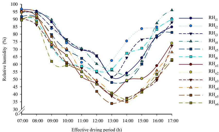
**Figure 4.** Relative humidity (%) as function of effective drying period in the solar collector: RH<sub>n</sub> – Relative humidity; i – inlet; m – middle; o – outlet; n – drying day.
