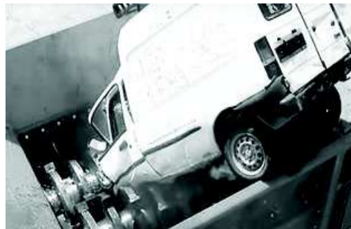
Figure 6. Cars rest is grinding without dismantling.
