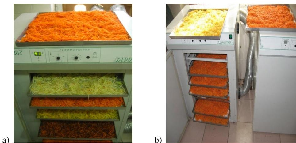
**Figure 2.** A general view of the convective dryer: a) carrot quantities prepared and loaded into the dryer's chamber; b) dried carrot quantities.
