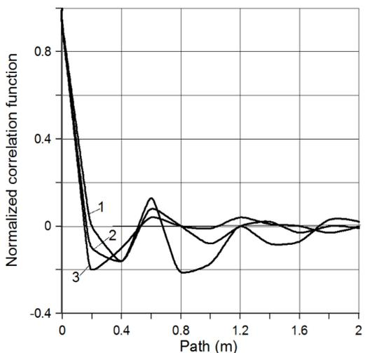
**Figure 7.** Normalized correlation functions of tillage depth oscillations at different operating speeds of combined tractor and harrow unit: 1) 2.1 m s<sup>-1</sup>; 2) 2.5 m s<sup>-1</sup>; 3) 3.3 m s<sup>-1</sup>.
