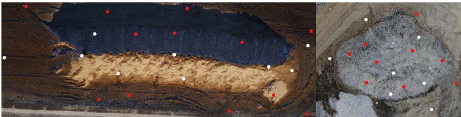
Figure 2. On the left an orthophotomosaic of the peat stockpile in Laiküla and on the right an orthophotomosaic of the selected object in Karude quarry. On the left special photogrammetric GCP's are marked with white and spray painted GCP's are marked with red dots. On the right the selected seven GCP's are marked with white and selected nine GCP's are marked with red dots.
