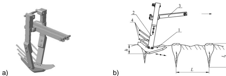
**Figure 1.** 3D model (a) and design and process schematic model (b) of vibrational lifting tool for sugar beet roots: 1 – digging shares; 2 – posts; 3 – kinematic tie link between posts and vibration generation device; 4 – extension pins.
