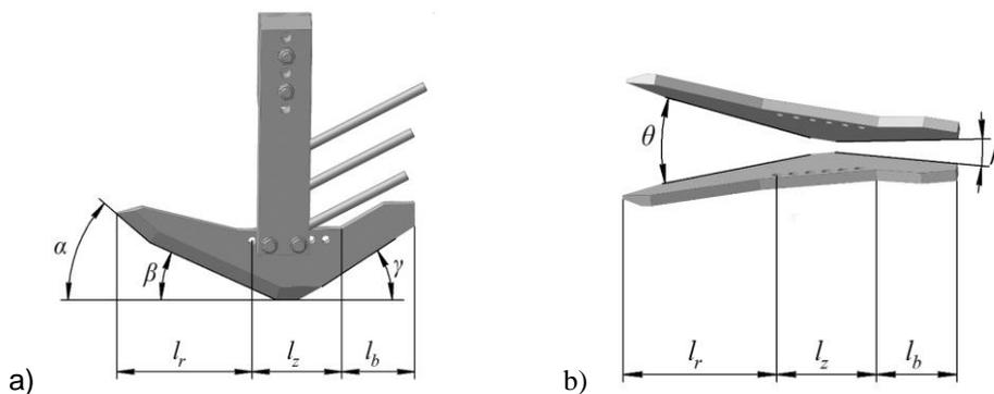
**Figure 2.** Structural dimensions of digging share (a) and working throat (b) of vibrational lifting tool.
