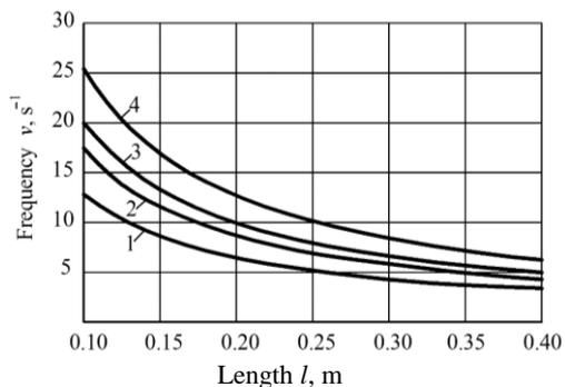
**Figure 4.** Relation between minimum permissible frequency  $\nu$  of oscillations performed by vibrational lifting tool and length  $l$  of its working throat rear part at following values of tool's translational motion velocity: 1)  $V = 1.30$  m s<sup>-1</sup>; 2)  $V = 1.75$  m s<sup>-1</sup>; 3)  $V = 2.00$  m s<sup>-1</sup>; 4)  $V = 2.55$  m s<sup>-1</sup>.
