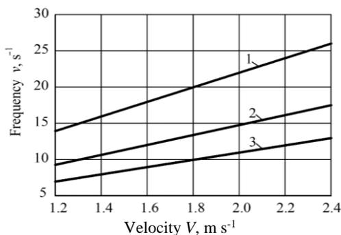
**Figure 3.** Relation between minimum permissible frequency  $\nu$  of oscillations performed by vibrational lifting tool and velocity  $V$  of its translational motion at following values of length of working throat rear part: 1)  $l = 0.10$  m; 2)  $l = 0.15$  m; 3)  $l = 0.20$  m.
