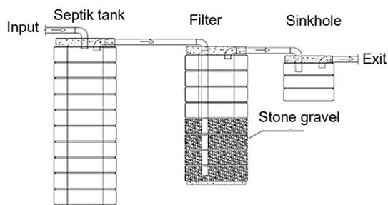
**Figure 1.** Section of the septic tank-filter-sinkhole of tires.
