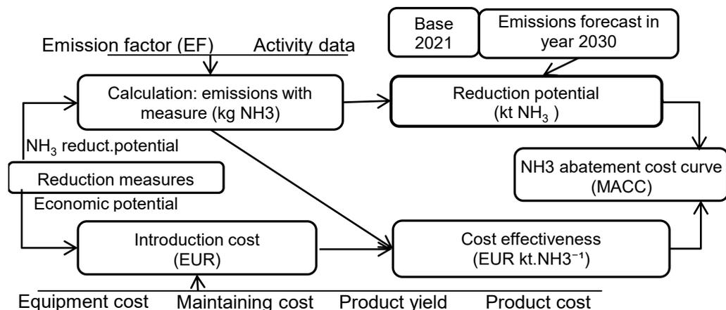
**Figure 1.** Model of an algorithm for calculating the marginal abatement cost of an NH<sub>3</sub> emission reduction measure and constructing a MACC curve.
