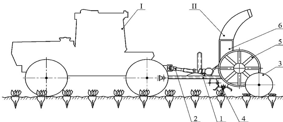
**Figure 1.** Design and process scheme of asymmetric top harvesting unit in longitudinal-vertical plane: I – wheeled tractor; II – trailed asymmetric harvesting machine; 1 – frame; 2 – universal-joint drive; 3 – pneumatic support-and-finder wheel; 4 – rotary haulm cutting device; 5 – conveying device; 6 – loading device.
