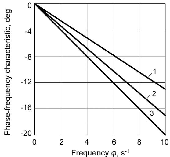
**Figure 5.** Phase-frequency characteristic of the course angle  $\varphi$  of the tractor of the integral configuration when it works out disturbances in the form of oscillations of the tiller turning angle  $\beta$  at different speeds of the machine: 1)  $V_o = 1.5 \text{ m s}^{-1}$ ; 2)  $V_o = 2.0 \text{ m s}^{-1}$ ; 3)  $V_o = 2.5 \text{ m s}^{-1}$ .
