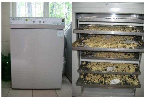
Figure 3. General appearance of chamber-type convection dryer with onion test samples in the process of drying. Power supply of drier: 220 V, 50 Hz, power rating - 1,250 W. Fresh onion batch load is 18 kg, at one tray load of 2 kg. Maximum temperature in process chamber - 65 \pm 5 °C. Control of drying conditions is semi-automatic.
