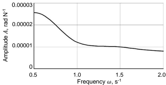
**Figure 4.** Experimental amplitude-frequency characteristic of fluctuations of the heading angle  $\varphi$  when the agricultural vehicle is working out the difference in tangential forces, applied, respectively, to the wheels of its left and right. Sides.
