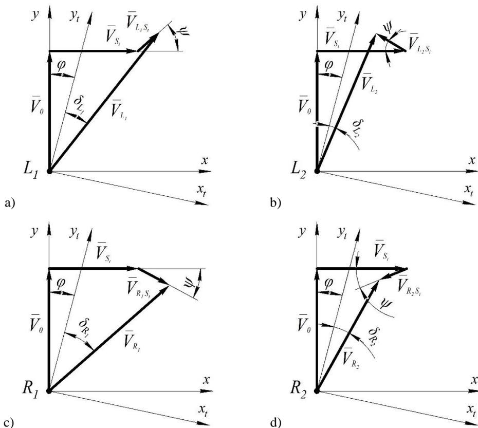
**Figure 3.** The vector sums of the speeds of the centers of the wheels of the wide span agricultural vehicle: a) – the front wheel of the left side with center  $L_1$ ; b) – the rear wheel of the left side with center  $L_2$ ; c) – the front wheel of the starboard side with center  $R_1$ ; d) – the rear wheel of the starboard side with the center  $R_2$ .
