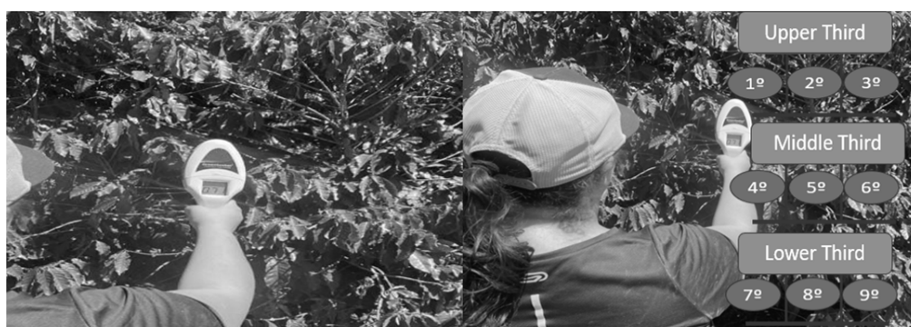
Figure 3. NDVI data sampling using the active sensor.
