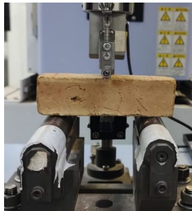
Figure 2. Three-point flexural test.
