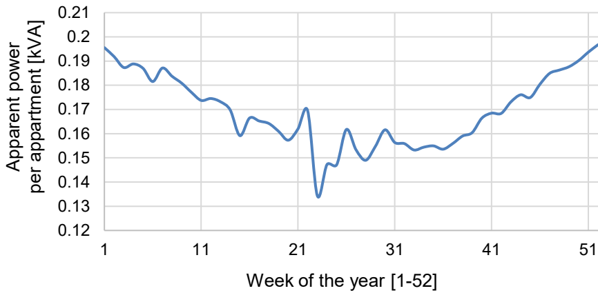
Figure 3. Average weekly apparent power consumption (kVA) per apartment by week number (1–52), reflecting seasonal variations. The curve includes a sinusoidal approximation based on fitted historical data.
